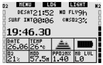
The remaining desaturation time (DESAT) is calculated by the decompression model in the computer. Any dive started while there is remaining desaturation on your computer is considered a repetitive dive, meaning that Galileo accounts for the pre-existing nitrogen load in your body.
