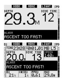
Galileo also provides an audible alarm in case of ascent rates exceeding 110%: the intensity of the alarm increases in direct proportion to the degree that the ideal ascent rate is exceeded.
