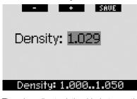
There is a direct relationship between the weight of a water column and the pressure exerted by it, and the weight is given by the depth multiplied by the density of the water. Hence, the depth displayed by a dive computer is obtained by a measurement of absolute pressure.
