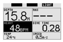
Galileo can trigger an alarm if your heart rate\* drops below a set level. The alarm can be set between 35 and 100bpm in 1bpm increments. If your heart rate\* drops to the level set in the alarm, a continuous beeping sequence goes off, and the heart rate\* is displayed in inverted colors (white on a black background).
