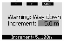
Galileo allows you to set a depth increment warning, so that during your descent (WAY DOWN), ascent (WAY UP), or both (BOTH), you can keep track of your progress without looking at the display. The warning can be set in 1m/5ft increments between 5m/20ft and 100m/330ft. Every multiple of the set interval, Galileo will trigger a 2-second audible sequence, consisting of two short beeps.
